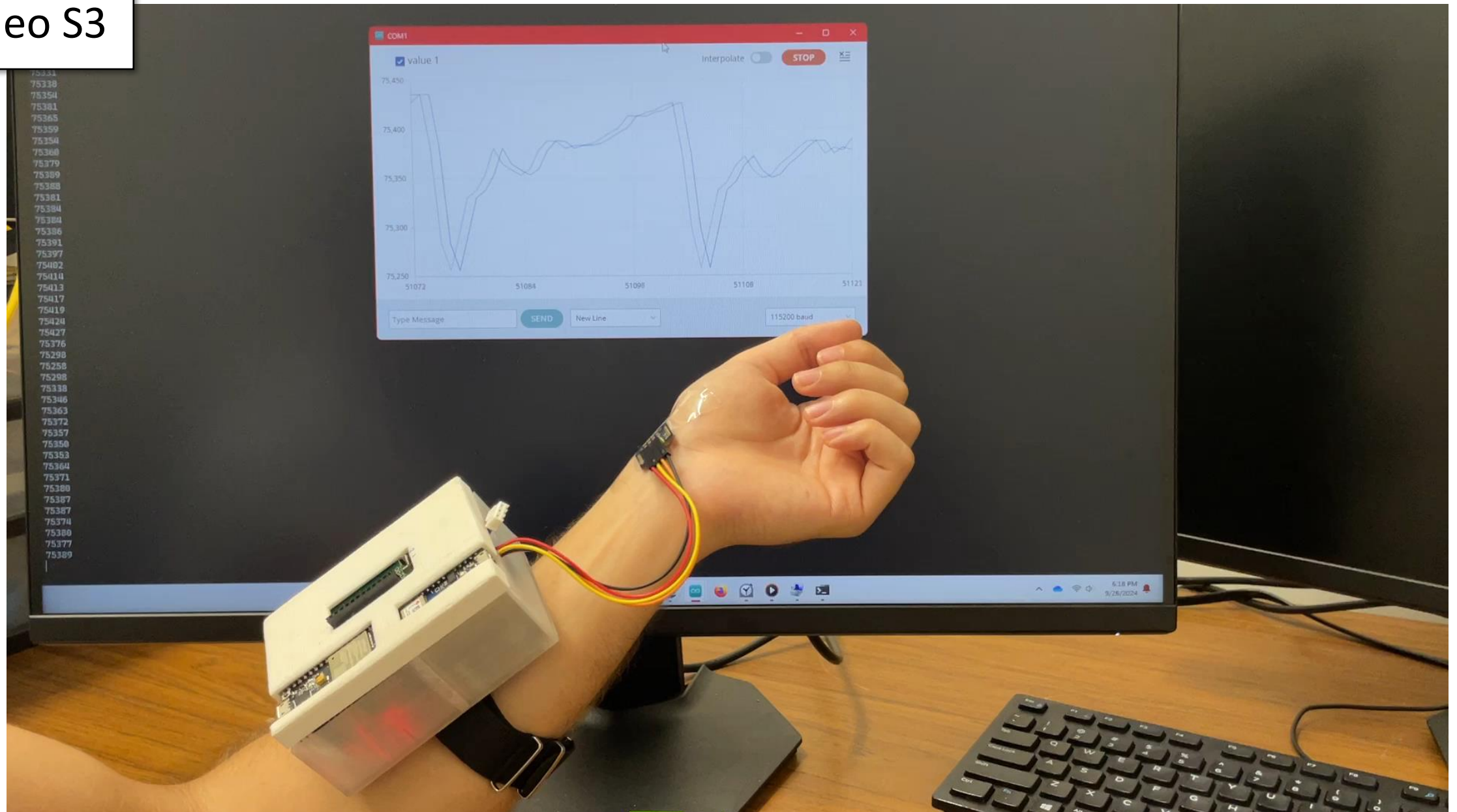
Video S3. Video demonstrating the induced noise caused by the proximity of IR radiation. The device, an MH-Sensor-Series IR obstacle detector, generates pulsating (5 Hz) IR radiation.
