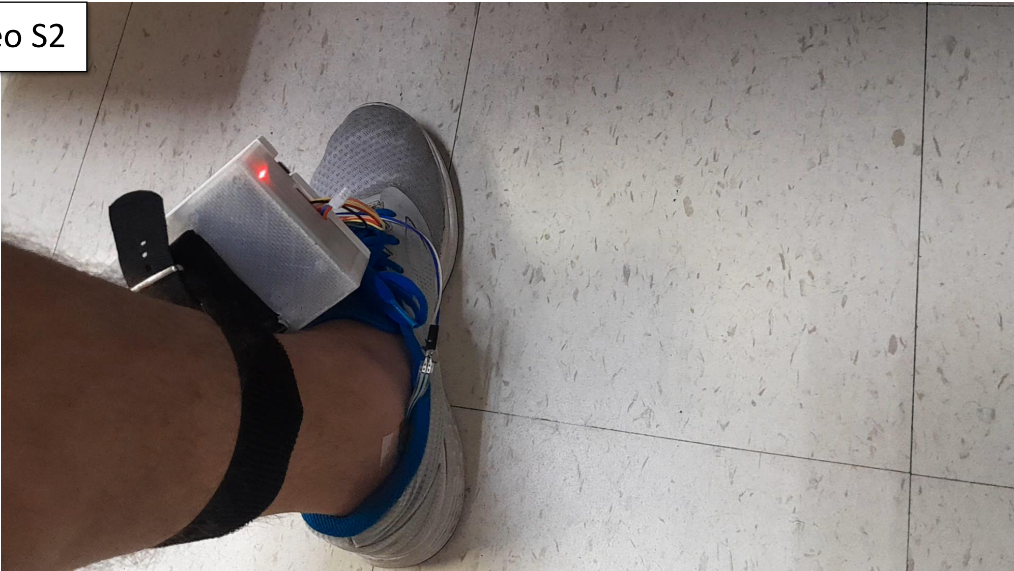
Video S2. Dual piezoresistive sensor on the ankle, capturing pulse waveform and transmitting data to the computer in real time.
